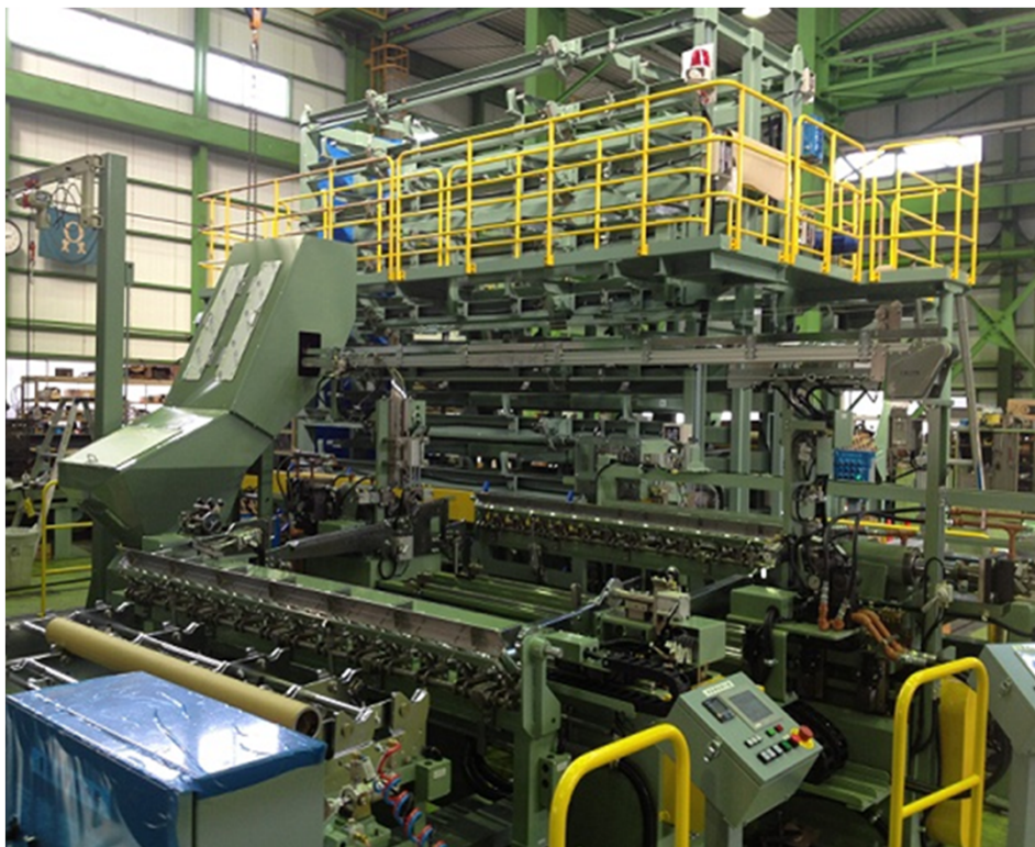
Core is manufactured according to the production order of the winder.
